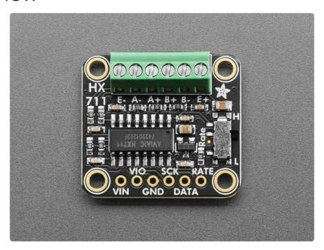
If you are feeling the stress and strain of a Wheatstone bridge and you want to quantify it, this handy breakout will do the job, no sweat! The **Adafruit HX711 Breakout** contains a super-high-resolution 24-Bit differential ADC with extra gain circuitry that makes it perfect for measuring strain gauges / load cells or other sensors that have four wires that are connected in a <a href="Wheatstone bridge arrangement">Wheatstone bridge arrangement</a> (https://adafru.it/-kd).
