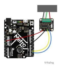
Strain gauge power to breakout E+ (red wire)
